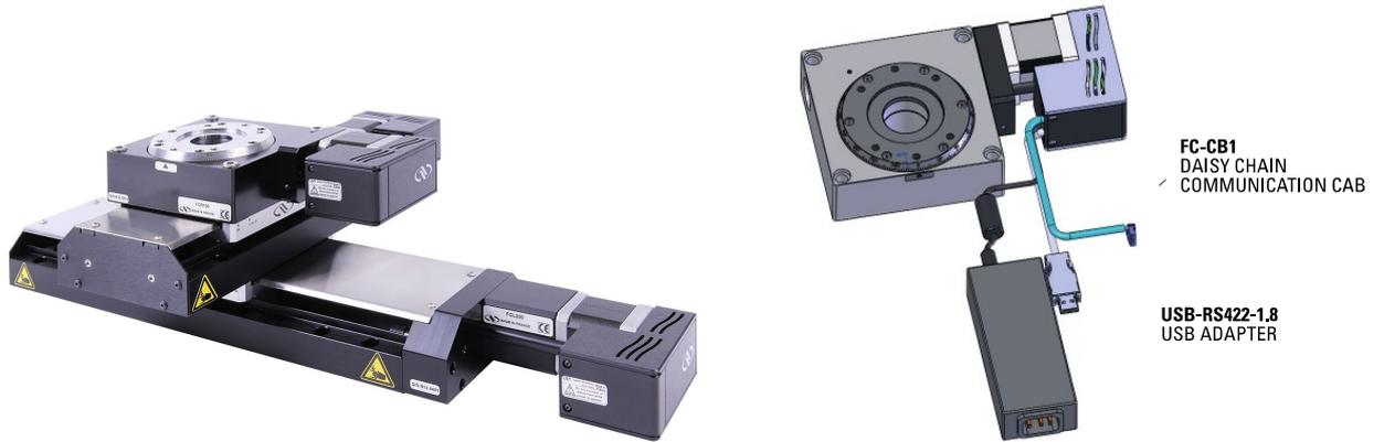
Once the controller address of each stage is set, unplug all the power cables and disconnect the USB cable from all the stages except for the FC controller that has its address set to 1. Use the daisy chain cables to connect each controller. For stages #2 thru 4, it does not matter whether you use the upper or lower RS422 connector to daisy chain.
